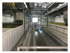
New this season was an additional hop kiln with automated fans and burner configurations paired to balance air delivery for drying hops. Advanced monitoring arms read temperature and moisture levels to help regulate applied air from fans, ensuring an even temperature across each hop bed. In addition is an automated storage bin mechanism that will be used to regulate moisture levels, improve baling processes, and ensure product quality.
