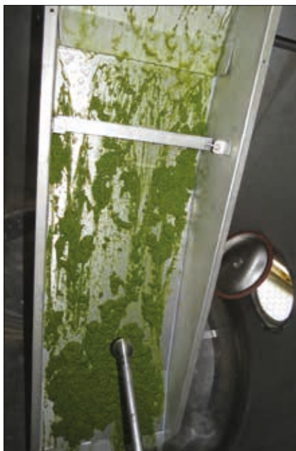
Fig. 2: Hops particles being separated in the Beer Cleaner
