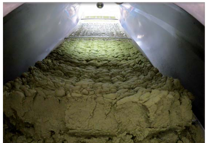
Fig. 4 Bottom discharge of hop trub
